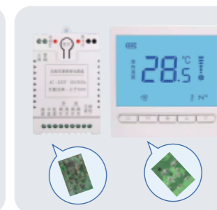
The Cooling/Heating Temperature Control Board
